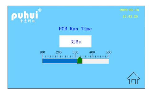
By dragging the ruler slider left and right to change the PCB run time, the run speed of the belt can be changed.
