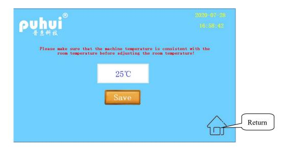
To calibrate the temperature of the machine, input the current room temperature in the dialog box when the internal temperature of the machine is consistent with the room temperature, click "save" to finish the room temperature calibration, and click the back button to enter the main menu interface.
