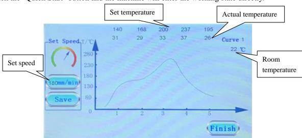
To adjust the welding speed, click the welding speed setting button to enter the setting interface. To discard the changes, click the "CLOSE" button. Adjust the welding speed by dragging the slider left and right to change the percentage. Click "OK" to exit the interface, and then click "Save" to adjust the welding speed. After welding, click the "Finish" button, and the machine will return to the main interface.
