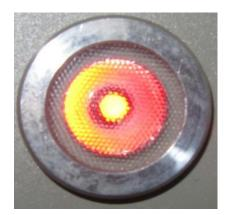
When the status indicator lamp shows red, it indicates that the main control board program is in running state; when the status indicator lamp shows green, it indicates that the main control board program is in setting state.
